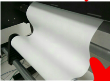
Fig. 2 Charging the HEXIS media in the printer
