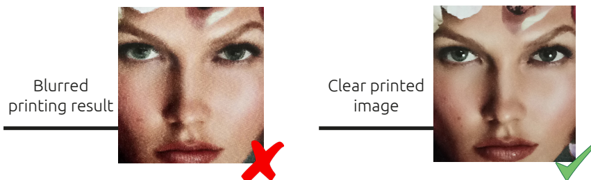
Fig. 17 Printing lag between an adjusted and an incorrect bidirection
