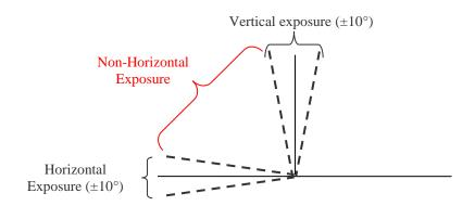
• The real durability of a product depends on a large number of parameters, including, among others, the quality and the preparation of the substrate, the exposure (environment, climate, exposure angle), the film maintenance, and the degree of pollution.
